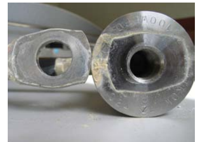
WEB 0 and cable lug after saltspray test
